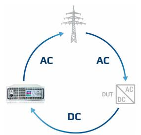
Operation of these recovering loads in terms of power generation is not intended. Grid protection devices, which could supervise the feedback of energy into the public grid, are available on the market for optional installation and are intended to achieve additional safety of persons and equipment, especially when running the so-called isolated operation.
